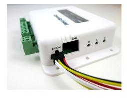
wired the same way as before: one wire from each valve should come together and go to the **COM** terminal on the OSBo; and the other wire from each valve goes to an individual station terminal.
