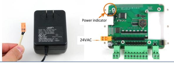
**Warning:** if the LED doesn't light up, please unplug the power immediately. If you can't figure out the problem, send an email to <a href="mailto-support@opensprinkler.com">support@opensprinkler.com</a>.
