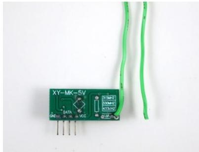
RF receiver with solder-on wire antenna
