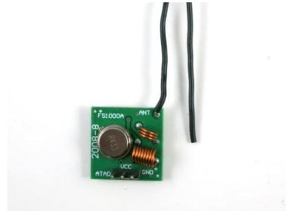
Transmitter with solder-on wire antenna
