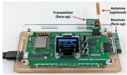
**Both the transmitter and receiver should be plugged in** <u>facing up</u>. If you use your own transmitter and receiver, you should verify the orientation by checking that the GND pin on the transmitter and receiver match the GND pin on the silkscreen printed next to the pin headers.
