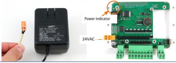
**Warning:** if the LED doesn't light up, please unplug the power immediately. If you can't figure out the problem, send an email to <a href="mailto:support@opensprinkler.com">support@opensprinkler.com</a>.
