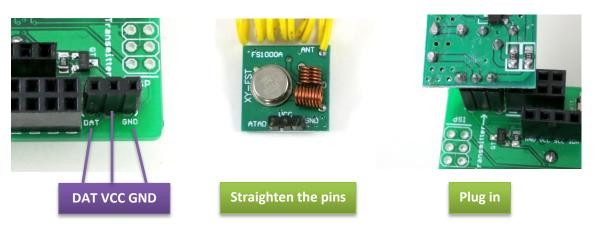
**NOTE**: Some transmitters may have different pin orders. For example, one of SparkFun's transmitters uses this pin order: GND, DAT, VCC. In this case, you can make use of the GND pin on the nRF24L01 header to match the pin order:
