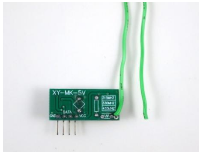
RF receiver with solder-on wire antenna
